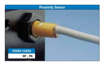
This L.E.D. device senses end-of-stroke with one of two normally open inductive d.c. proximity sensors. NPN supplies a sinking signal; PNP supplies a sourcing signal to a device such as a programmable logic controller.
