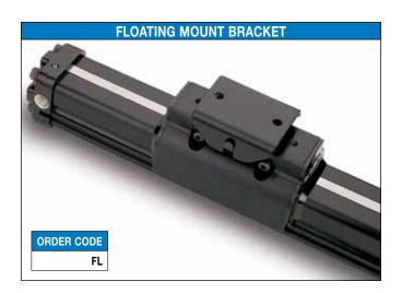
For applications where a BC2 band cylinder is moving a load that is externally guided and supported. An externally guided load, not parallel to the BC2 band cylinder may result in cylinder binding. The floating mount bracket compensates for nonparallelism between the cylinder and the external guide.
