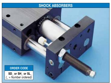
Magnetically coupled slides with standard internal bumpers offer an effective method of decelerating loads. However, magnetically coupled slides are capable of carrying heavier loads at higher velocities than the internal bumpers can absorb. Optional shock absorbers can be used to increase the unit's life and broaden the application range for the magnetically coupled slide you have chosen.
