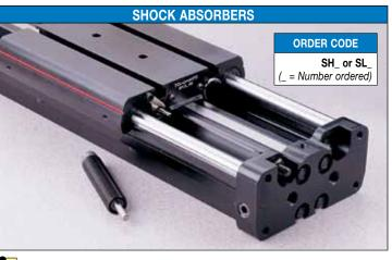
Rodless cylinders with standard internal cushion offer an effective method of decelerating loads. However, all Tolomatic rodless cylinders are capable of carrying heavier loads at higher velocities than the cylinder cushion can absorb. Optional shock absorbers can be used to increase the cylinder's life and broaden the application range for the cylinder model you have chosen.
