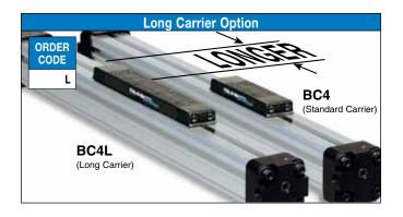
Long carrier option greatly increases the "My" and "Mz" moment load capacity. This broadens the application range for these models. Other benefits include larger mounting surface and virtual elimination of chatter for vertical cantilever loads.
